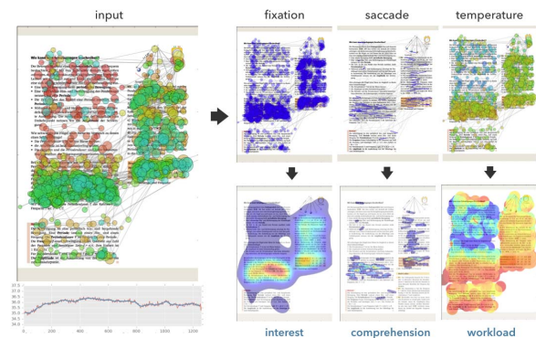
Fig. 1. The key idea of our work. Combining eye tracking and thermography to recognize cognitive states while learners are reading a document.
